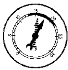
POOR VALVE SEATING AT IDLE
