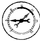
BLOWN HEAD GASKET AT IDLE
