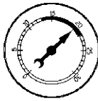
NORMAL READING RANGE AT IDLE
