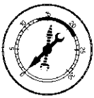
RESTRICTED EXHAUST (DROPS TOWARD ZERO AS ENGINE RPM INCREASES)
